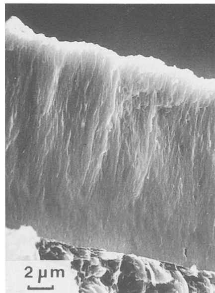
Figure 12 Fracture surface of a 15 \mu\text{m} thick SiC coating deposited at 1573 K.
